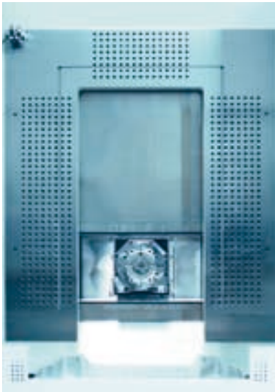
FM 3+X basis frame mounts the work piece specific configuration and the C-axis
