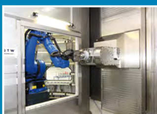
SMX 5181 Automatic tool change by robot
