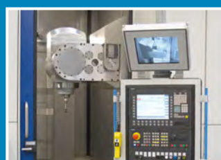
SMX 5181 Swivable work area camera monitoring system
