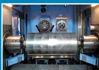
SPX 5111 Work area with clamped printing cylinder
