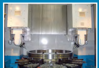
RTX 5135 Vertical 2 spindle machining with H/V-milling head
