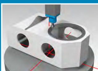
Vertical surface machining: 3-axes interpolation with vertical milling head
