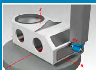
Vertical surface machining: 4-axes interpolation with horizontal milling head
