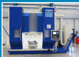
RTX 5280 Vertical 2 spindle machining of perforated discs
