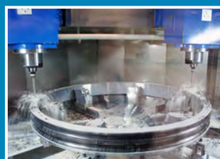
RTX 5211 Vertical 2 spindle machining of large scale bearing rings
