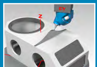
Free form shape machining 5-axes simultaneous machining with HV head, dynamic B-axes
