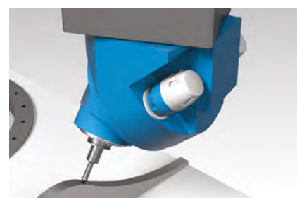
5-axes simultaneous machining with HV head, dynamic B-axis
