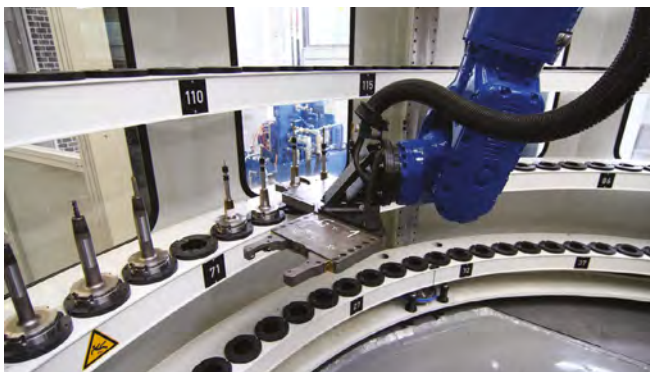
Tool Arena with tool change robot
