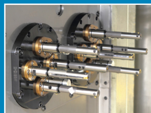
Examples of multispindle heads used in ELHA FM production modules.
