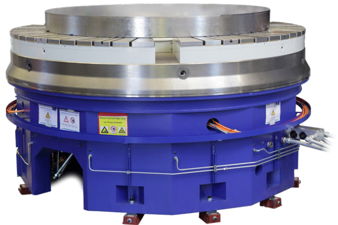
[3] The ELHA-SSD (Segment Direct Drive) table drive concept developed in-house, based on the principle of a magnetic levitation train, is proving to be a secret weapon in the context of high-precision finishing of expensive large components
