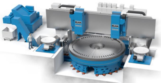
Vertical turning milling center VTM 602 *ht*
